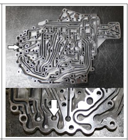
18. Punch center of hole using a center punch.
