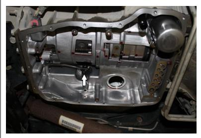
31. Torque the valve body attaching bolts to 105 in/lbs.
