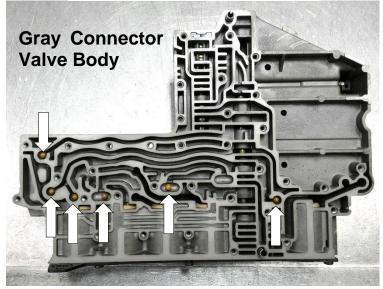
23. Install the BD bonded gasketed separator valve-body plate (1600188).
