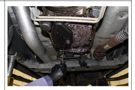
11. Remove the six 8mm bolts securing the valve body to the transmission. Drain valve body of fluid. To remove valve body from transmission, wiggle it while pulling downwards to work the electrical connector through the case.
