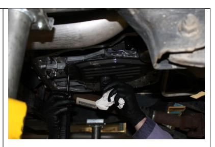
33. Place the supplied gasket on the transmission pan. Hold pan below transmission and install attaching screws. Torque the pan screws to 105 in/lbs.
