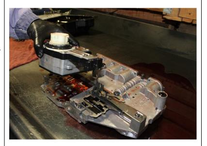
14. Remove remaining thirty-five T25 Torx screws securing the valve body halves.
