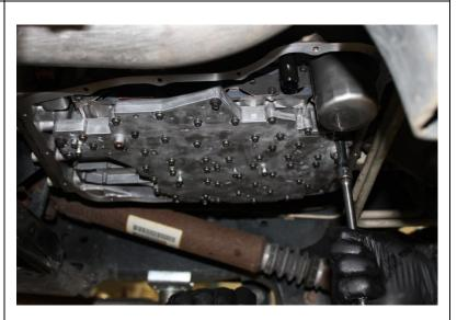
32. If desired, install new filter(s). Otherwise, reinstall the filter/pickup assembly. Torque to 50 in/lbs.
