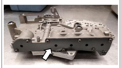
28. Inspect the three rubber seals on the top of the valve body, replace with supplied seals if they are nicked or otherwise damaged. Ensure the seal mating surface on the transmission is clean.
