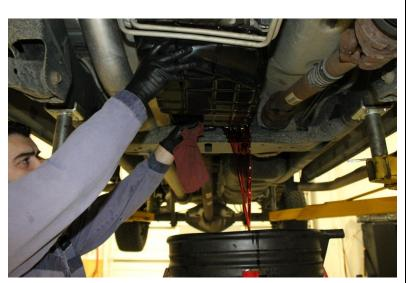
10. Remove transmission filter by removing the one T25 Torx screw.
