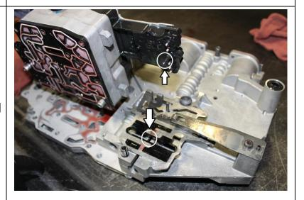
IMPORTANT! – On rare occasions, the solenoid pack gasket comes with a small nub on one side which will need to be removed using a file or blade before installation as the new plate blocks off the opening as it is not present on most applications.
