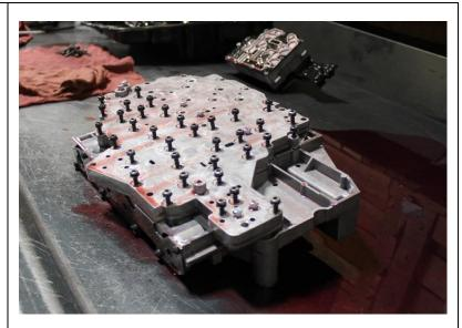
15. Carefully separate the two halves of the valve body. Separate as shown in pictures – do not invert the larger (top) portion as it contains plastic check balls. The two halves will have to be wiggled apart as the alignment dowels will be holding them together.
