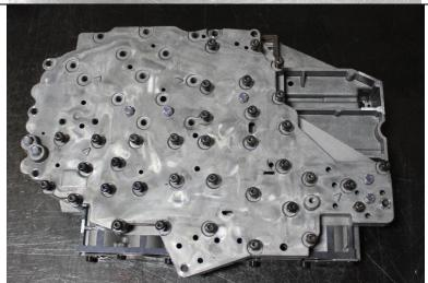
25. Re-install solenoid pack onto valve body. Be sure to properly align the pin on the solenoid pack with the slot on the valve body. Due to the alignment dowels, the valve body may need to be wiggled down into position. Install solenoid pack attaching screws. Install remaining Torx screws to fasten the solenoid pack to the valve body.
