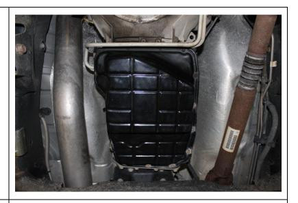
9. Tap pan with a mallet to break the silicone gasket seal. Allow fluid to drain. Remove last screw and drain remainder of fluid.
