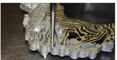
19. Drill hole with 1/8" drill bit.
