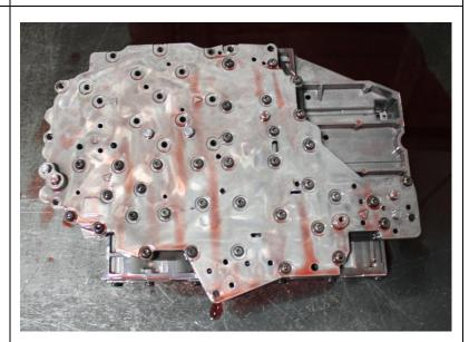
13. Remove fifteen T25 Torx screws securing the solenoid pack to the valve body, remove solenoid pack and place it to the side.
