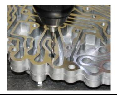
20. Thoroughly remove any burrs and clean all shavings from the valve body. It is imperative that no contaminates are left as they may cause transmission damage.
