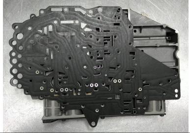
24. Re-install bottom (smaller) half of valve body. Ensure it fits flat on the separator plate/gasket. It may need to be worked downwards while rocking to be installed over the dowels. Install attaching screws so they are fully seated but do not tighten until the solenoid pack has been installed.
