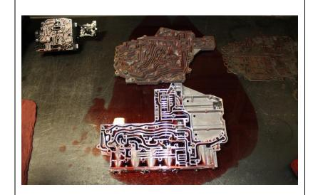
17. Thoroughly clean the bottom (smaller) half of the valve body. Locate the passage to be drilled.
